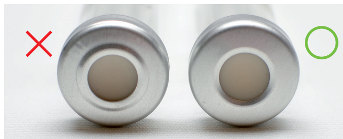
Figure 1. The vial to the left is capped too tightly.
