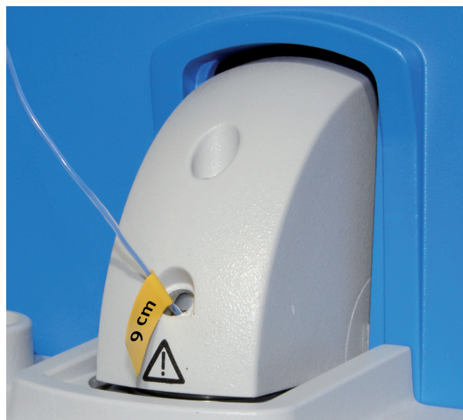
Figure 11. Insert a maximum of 9 cm of the probe when using 0.2–0.5 mL microwave reaction vials and 10 cm when using the other three reaction vials.
