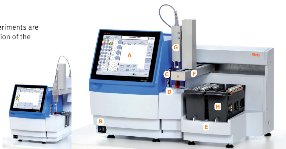
Figure 4. Left: Robot Eight. Right: Robot Sixty. A = touch screen, B = mains switch, C = cavity lid, D = cavity insert holder, E = robot, F = robot arm, G = gripper, and H = rack.
